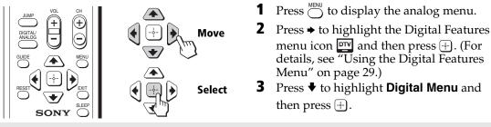
If the TV is in analog tuning mode, it will switch to digital tuning mode when displaying the digital menus.
